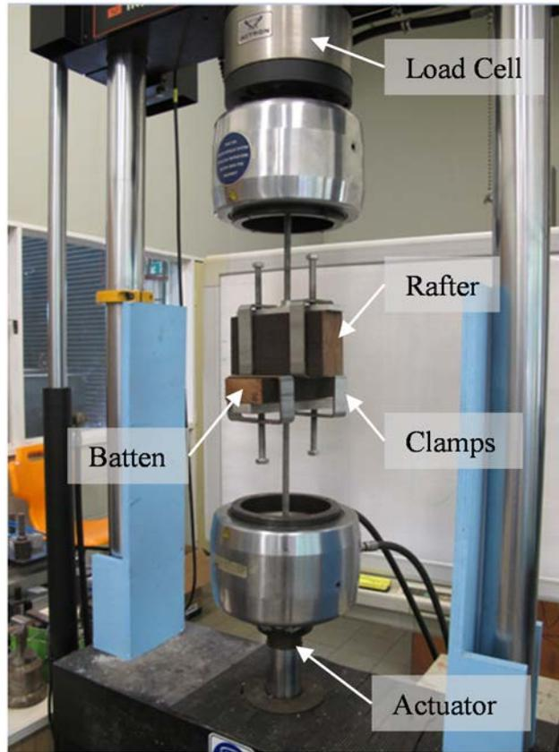
*Figure 4.2 Apparatus for static and dynamic connection testing*
