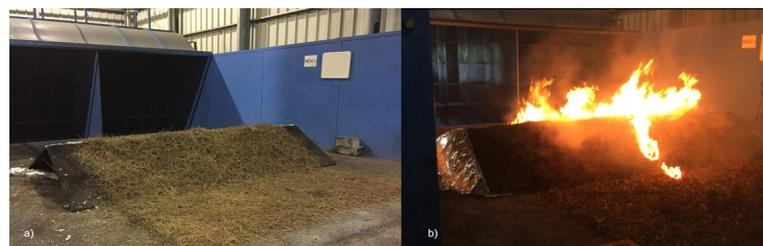
**Fig 2. Images from the TC 3 combustion wind tunnel used for the experiments.** (a) Example of model hill and fuel bed set up (note image was prior to installation of rounded ends on hill). (b) View of model hill (leeward slope) during an experiment with 2 spot fires. Combustion tunnel fan outlets are in the background in both images.
