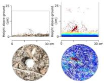
Figure 3. a) Point clouds captured using TLS and SfM techniques. b) plots showing dry weight against TLS and SfM estimate volume.
