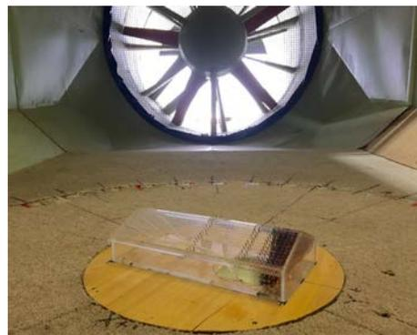
Fig 1: The 1/50 scale model in the Cyclone Testing Station boundary layer wind tunnel
