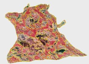
Figure 3: Implementation of the Super Iterative Linear Clustering (SLIC) segmentation method applied to the high resolution aerial imagery to delineate homogeneous areas prior to burn severity attribution.
