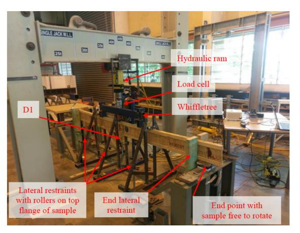
Figure 3: Four Point Bend Test Setup
