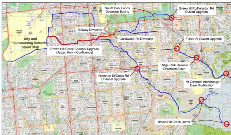
FIGURE 2. LOCATION OF FLOOD-CONTROL DAMS FOR OPTIONS B1 AND B2 (SOURCE: BHKCP, 2016)
