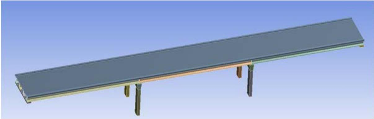
FIGURE : GEOMETRIC MODEL CREATED IN ANSYS (ELEVATION)
