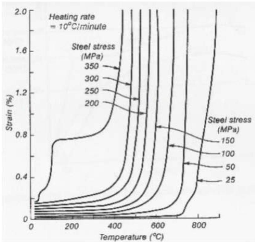
FIGURE 27: CREEP OF STEEL IN TENSION [107]
