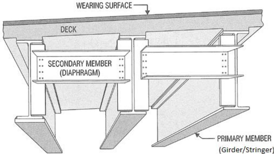
FIGURE 3: BRIDGE TYPICAL SUPERSTRUCTURE COMPONENTS [1]
