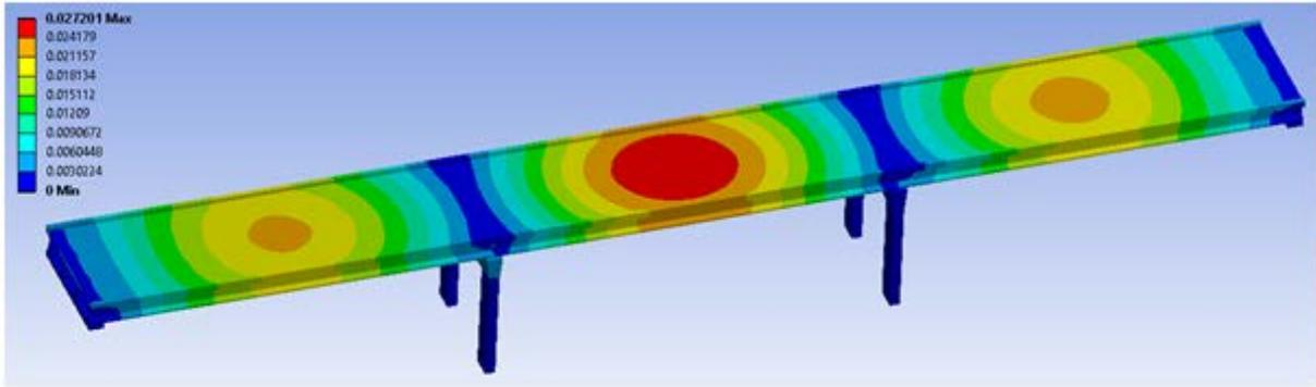
FIGURE 6: DISPLACEMENT CONTOURS OF THE BRIDGE DUE TO EARTHQUAKES
