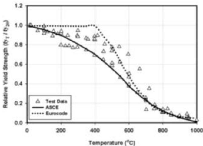
FIGURE 24: REDUCTION IN YIELD STRENGTH OF STEEL AT ELEVATED TEMPERATURES[101]
