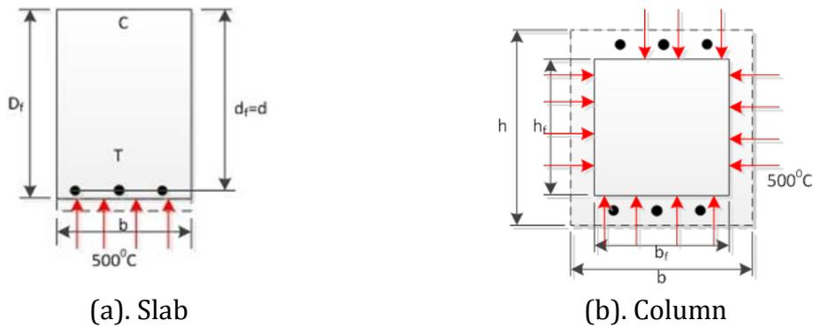
FIGURE 30: REDUCED CROSS SECTION OF REINFORCED CONCRETE MEMBERS
