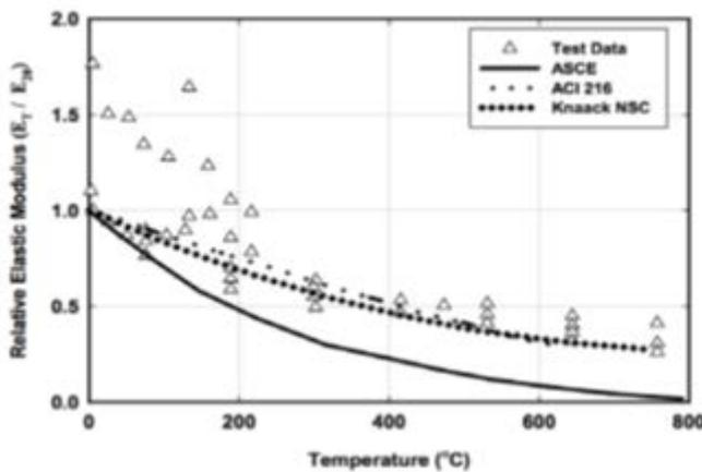
FIGURE 29: REDUCTION IN ELASTIC MODULUS AS TEMPERATURE RISES [101]
