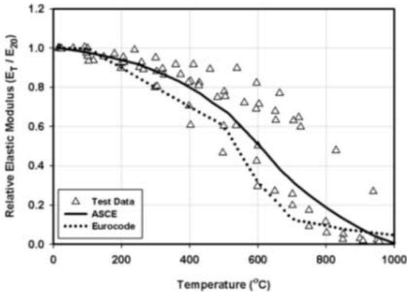
FIGURE 25: REDUCTION IN ELASTIC MODULUS OF STEEL AT HIGH TEMPERATURES[101]
