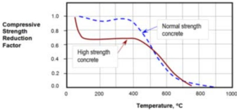
FIGURE 28: REDUCTION IN STRENGTH OF NORMAL STRENGTH AND HIGH STRENGTH CONCRETE IN HIGH TEMPERATURES [103]
