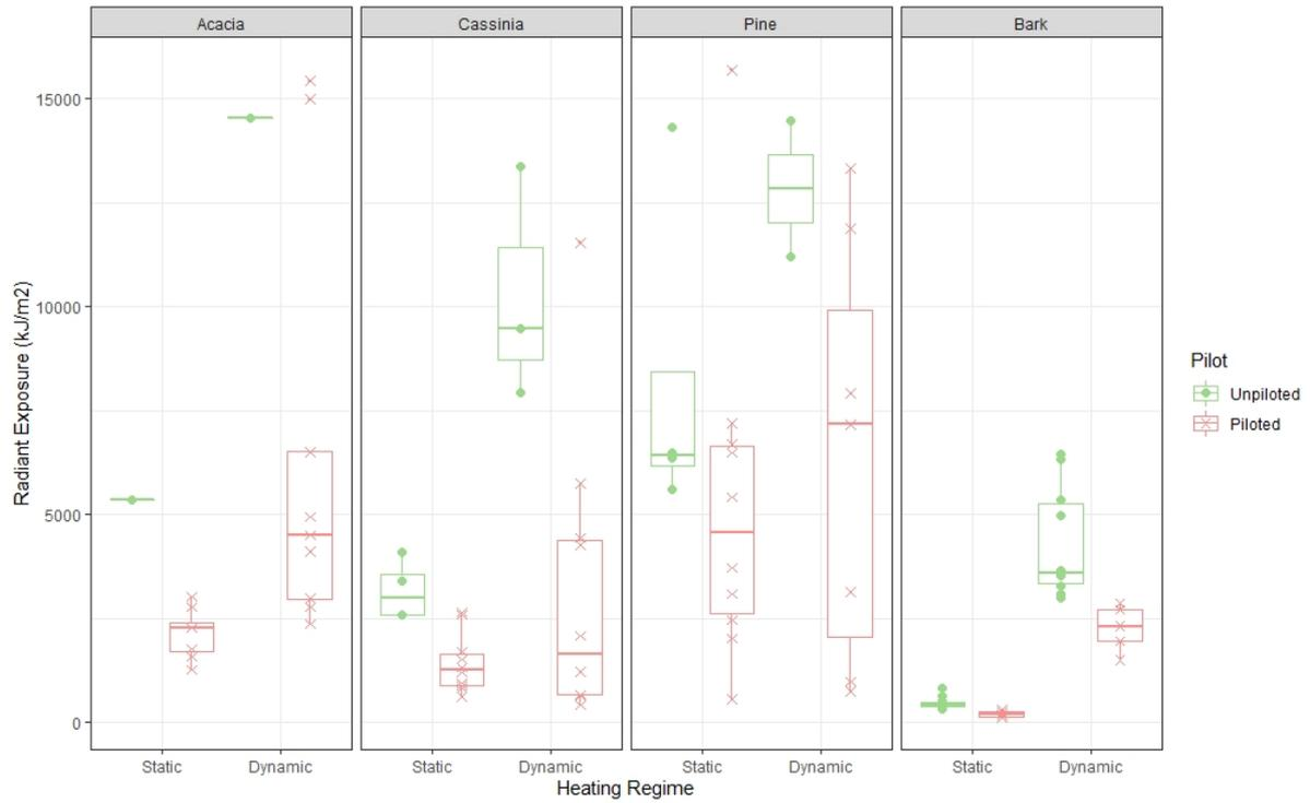
FIG. 6. RADIANT EXPOSURE/ $H_e$  (KJ/M<sup>2</sup>) AT FLAMING IGNITION COMPARING STATIC AND DYNAMIC HEATING REGIMES (X-AXIS) IN BOTH UNPILOTED (GREEN) AND PILOTED (RED) EXPERIMENTS.
