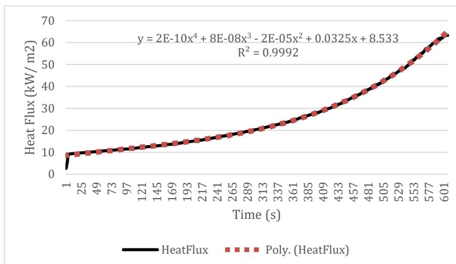
FIG. 4. DYNAMIC HEAT FLUX CURVE PRODUCED FROM CALIBRATION EXPERIMENTS AND FITTED WITH POLYNOMIAL FUNCTION.
