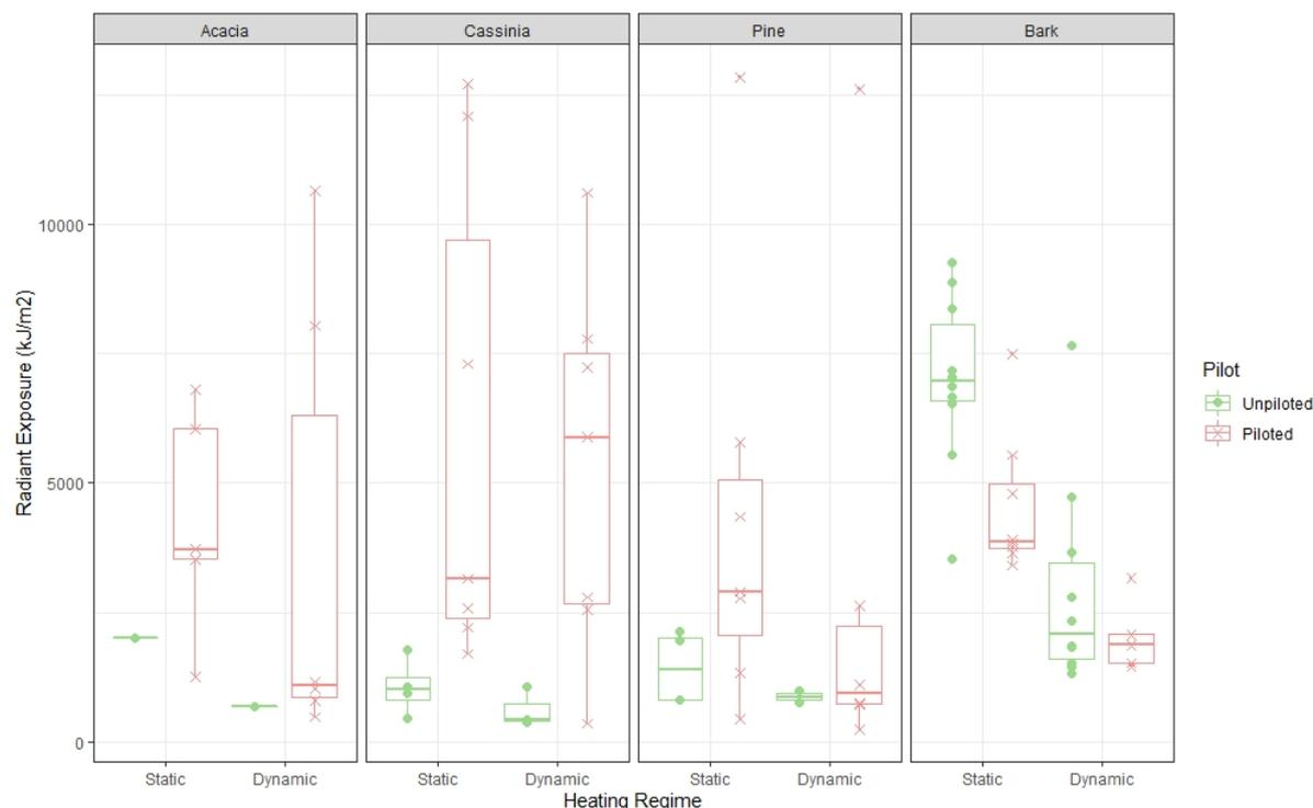
FIG. 8. RADIANT EXPOSURE/ $H_e$  ( $KJ/M^2$ ) BETWEEN FLAMING IGNITION AND COMPLETE CONSUMPTION (CONSUMPTION TIME) COMPARING STATIC AND DYNAMIC HEATING REGIMES (X-AXIS) IN BOTH UNPILOTED (GREEN) AND PILOTED (RED) EXPERIMENTS.
