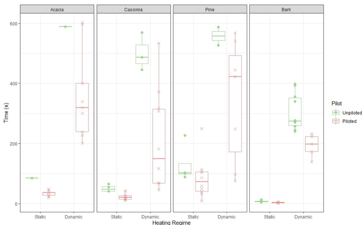
**FIG. 5.** TIME (S) TO FLAMING IGNITION COMPARING STATIC AND DYNAMIC HEATING REGIMES (X-AXIS) IN BOTH UNPILOTED (GREEN) AND PILOTED (RED) EXPERIMENTS.
