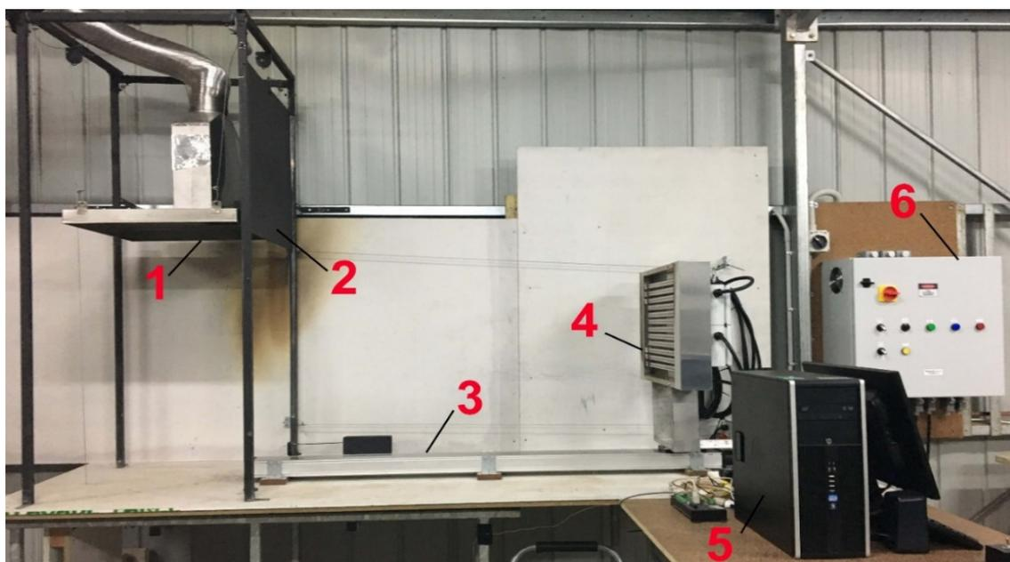
FIG. 2. VARIABLE HEAT FLUX (VHFLUX) APPARATUS 1) AN EXHAUST SYSTEM, 2) A SHUTTER, 3) A LINEAR STAGE, 4) A RADIATIVE PANEL, 5) A PC CONTROL SYSTEM AND 6) A POWER CONTROL BOX.
