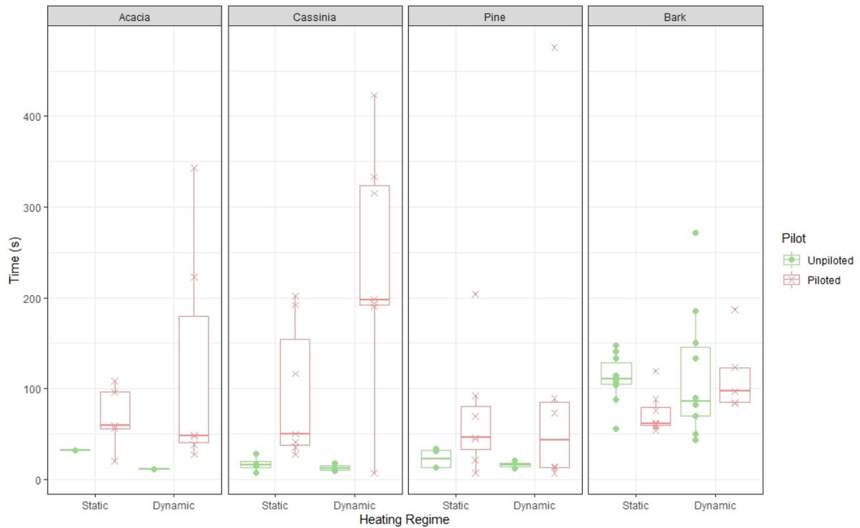
FIG. 7. TIME (S) BETWEEN FLAMING IGNITION AND COMPLETE CONSUMPTION (CONSUMPTION TIME) COMPARING STATIC AND DYNAMIC HEATING REGIMES (X-AXIS) IN BOTH UNPILOTED (GREEN) AND PILOTED (RED) EXPERIMENTS.
