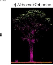
Airborne and ground-based LiDAR dataset complement each other very well since Airborne LiDAR captures the canopy whereas ground LiDAR accurately measures the ground and elevated fuels.
