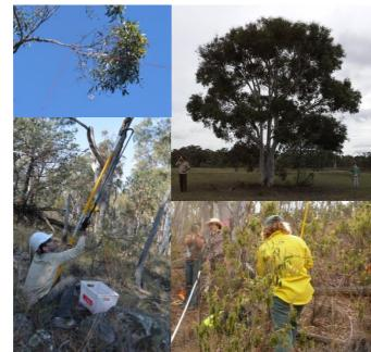
Ground based LiDAR (Zebedee) was collected to provide high resolution, reliable understory information useful to validate and/or complement airborne data.
