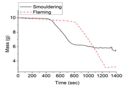
Figure 3: Mass loss profile for smouldering and flaming combustion. Initial mass: 10 grams.
