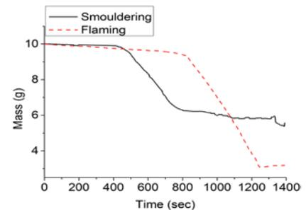
Figure 3: Mass loss profile for smouldering and flaming combustion. Initial mass: 10 grams.
