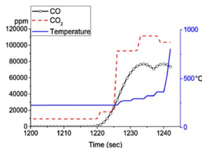
Figure 2: Temporal CO, CO<sub>2</sub> and temperature profile during the transition from no ignition to flaming combustion. Radiant heating flux = 11.2 kW/m<sup>2</sup>. Air flow rate = 7.0 grams/min.
