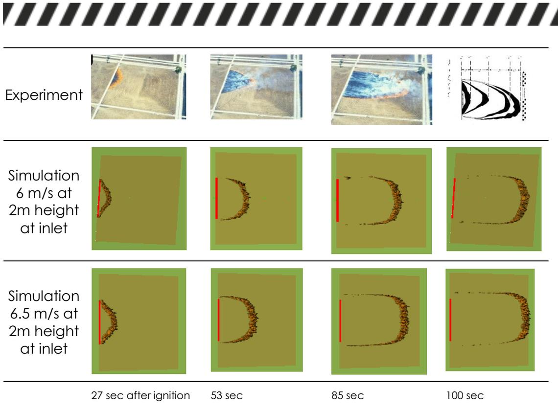
Figure 9: Model validation: fire propagation
