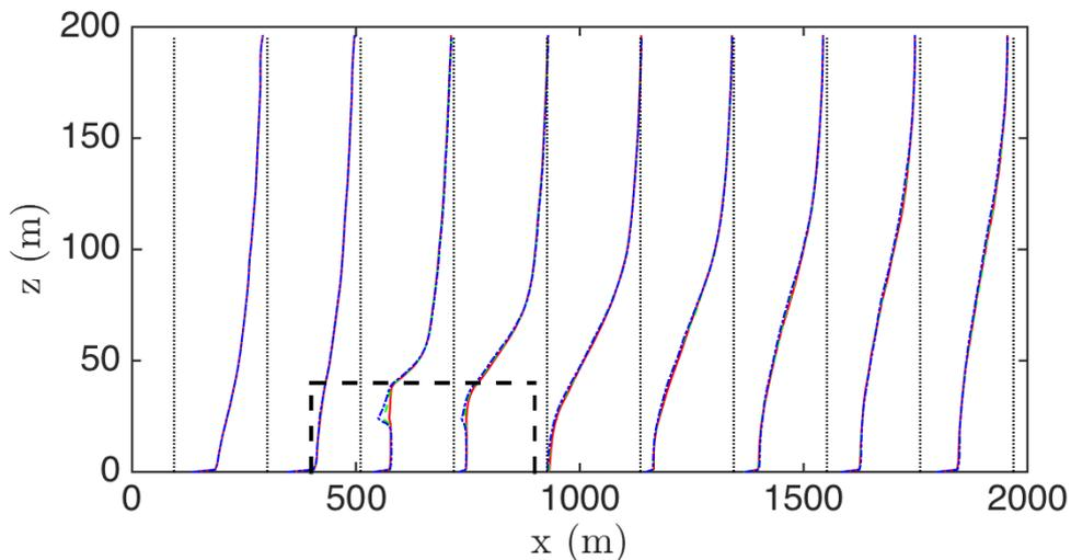
Figure 5: Variation in the average streamwise velocity profiles along 500 m canopies with variation in LAD. Red(solid):  $\max(\text{LAD}) = 0.2$ , green (dashed): 1.1, blue (dotted) 3.1. Note only the minor differences in the leafy crown region.
