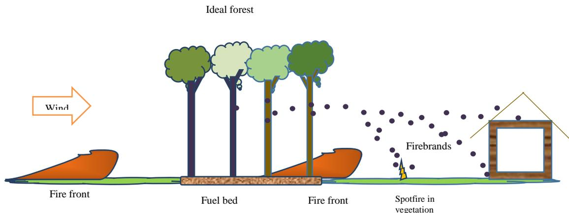
Figure 1: A schematic of fire spread mechanism in the ideal forest causing spotting in vegetation and house
