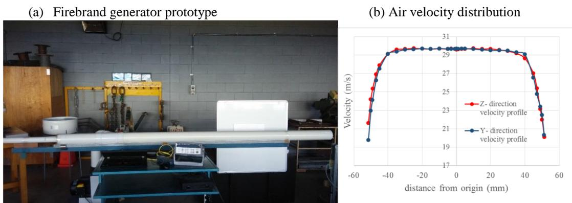
Figure 6: Firebrand generator prototype and air velocity distribution
