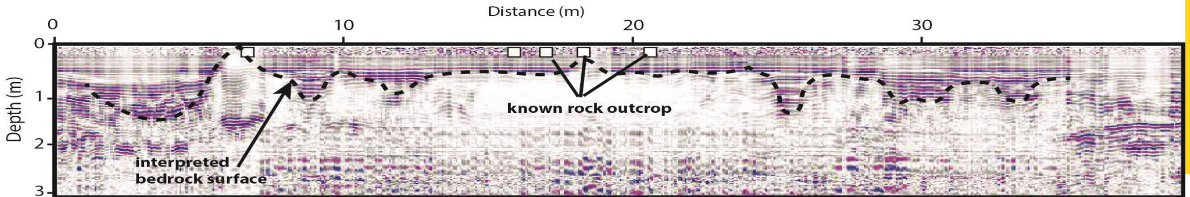
Ground Penetrating Radar Image of the Old Bar Sub-surface
