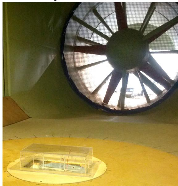
Wind Tunnel Set-up of Scale Model
