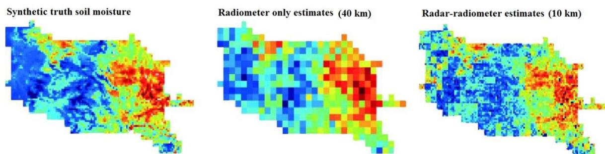
**Figure 5.** The comparison of synthetic ground-truth soil moisture with lower resolution (40 km) radiometer and the higher resolution (10 km) soil moisture estimates obtained from the active-passive method. The active and passive soil moisture retrievals are synthetically produced from an OSSE. Courtesy: Piles et al. (2009).
