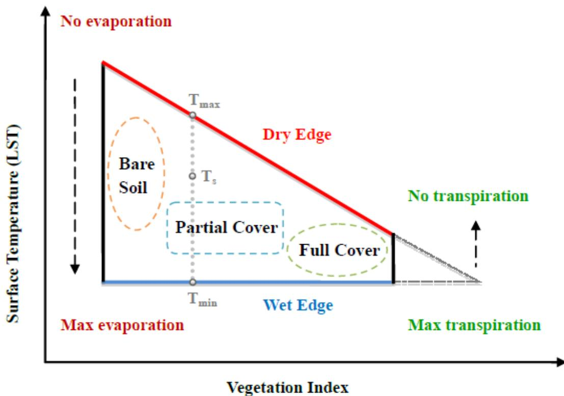
**Figure 3.** Conceptual diagram of the triangular/trapezoidal feature space that is constructed by land surface temperature and vegetation index (Courtesy: Pen et al., 2016).
