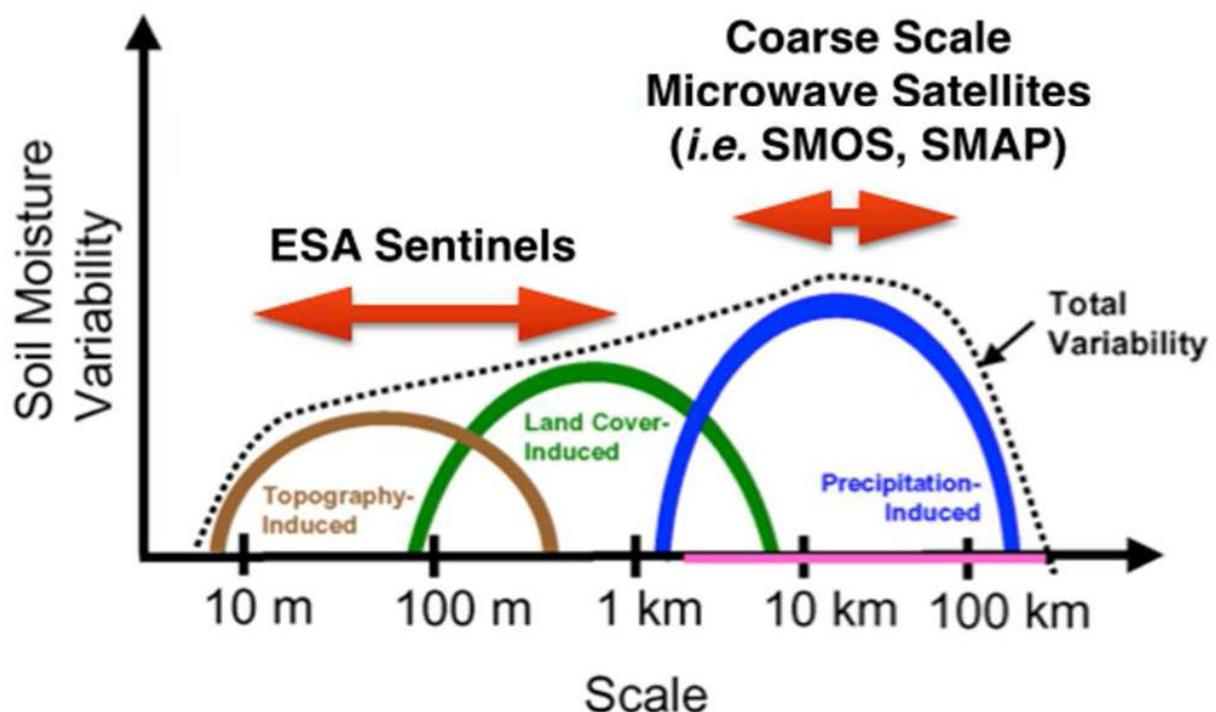
**Figure 6.** Diagram depicting the scales measured by different sensors and soil moisture spatial variability captured. Courtesy: de Jeu (2015).
