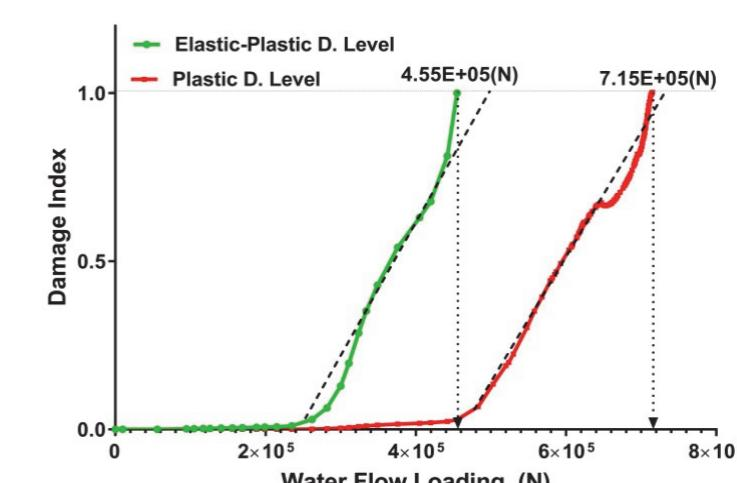
Damage evaluation for the whole system for different damage levels.
