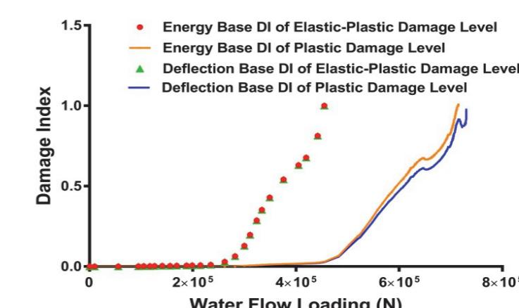
Damage Index for different damage levels and comparing the displacement and energy concept
