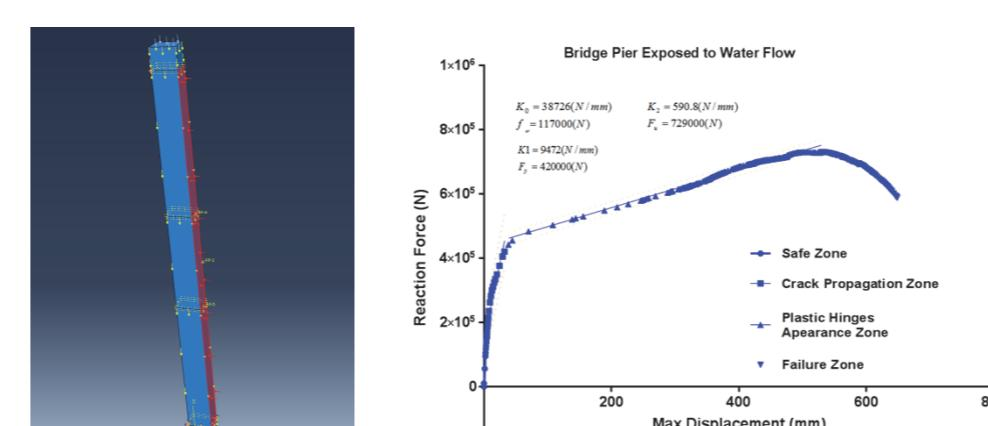
Configuration of different damage level based on load-deflection curve
