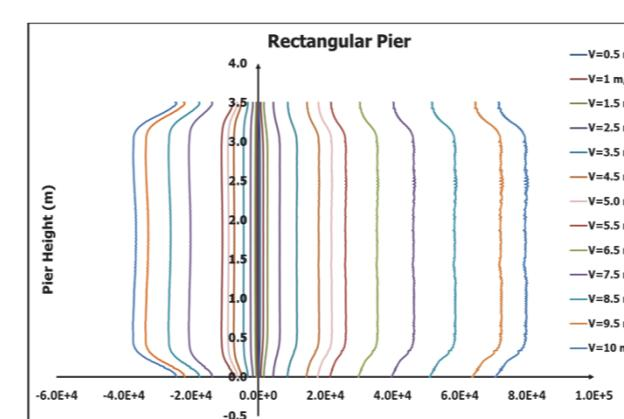
pressure distributions long the pier height in different water flow velocities
