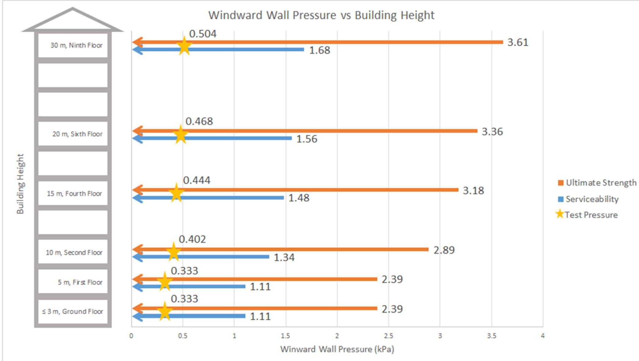
Relationship between ultimate strength design pressure, serviceability design pressure and the test pressure for the Australian Standard water penetration test (AS20147)
