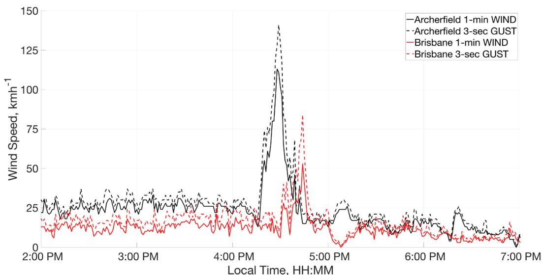
Figure 2: Archerfield and Brisbane AWS one-minute mean wind speed (WIND in km/h) and maximum three-second gust (GUST in km/h) wind histories. Measurements were collected on 27 November 2014 and time is shown in local standard time on the x-axes.
